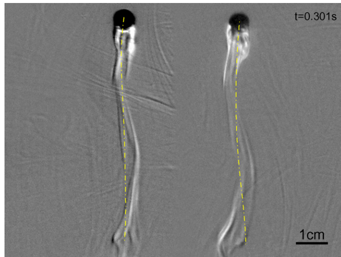
Fig. 13. Stereoscopic Schlieren image of the wake of a rising sphere in the ‘destroyed’ zigzagging periodic regime (case F). The picture was taken t = 0.301 s after the sphere had entered completely the field of view. Note the different character of the wake as compared to that shown in Fig. 12.
